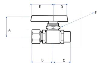
Kantleak<sup>™</sup> Instrumentation Ball Valves are designed with double O-ring stem seals to provide over 20,000 leak free cycles. These valves also feature an exclusive stem seal design that never needs tightening and can be panel mounted for instrumentation applications.
