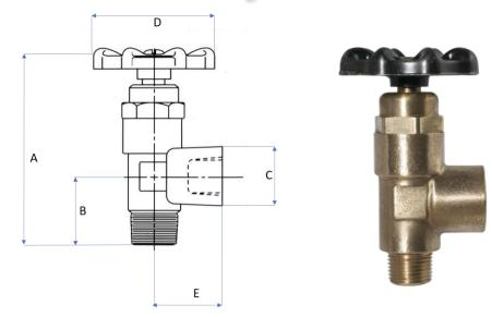
**900 Series** Rising Stem Valves are used extensively in the industrial, heavy duty construction equipment and mobile fleet markets. They are high flow valves recommended for operation with gasoline, oil, kerosene, LP gas, gas-air mixtures, cooling systems and air systems.
