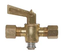
Instantaneous off-on operation with 360° rotation. The lapped brass body and plug are individually mated, providing an excellent quality, low friction valve. Valves are extensively used for water process piping and air supply systems.
